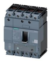
circuit breaker 3VA1 IEC frame 160 breaking capacity class S Icu=36kA @ 415V 4-pole, line protection TM240, ATAM, In=125A overload protection Ir=88A...125A short-circuit protection Ii=5...10 x In N conductor protection 100% clamp connection
