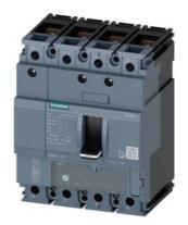
circuit breaker 3VA1 IEC frame 160 breaking capacity class S Icu=36kA @ 415V 4-pole, line protection TM220, ATFM, In=125A overload protection Ir=88A...125A short-circuit protection Ii=10 x In N conductor protection 100% nut keeper kit
