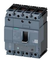
circuit breaker 3VA1 IEC frame 160 breaking capacity class S Icu=36kA @ 415V 4-pole, line protection TM240, ATAM, In=125A overload protection Ir=88A...125A short-circuit protection Ii=5...10 x In N conductor protection 50% nut keeper kit
