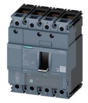
circuit breaker 3VA1 IEC frame 160 breaking capacity class S Icu=36kA @ 415V 4-pole, line protection TM220, ATFM, In=125A overload protection Ir=88A...125A short-circuit protection Ii=10 x In N conductor protection 50% nut keeper kit
