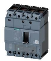
circuit breaker 3VA1 IEC frame 160 breaking capacity class S Icu=36kA @ 415V 4-pole, line protection TM240, ATAM, In=125A overload protection Ir=88A...125A short-circuit protection Ii=5...10 x In N conductor unprotected nut keeper kit
