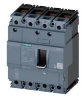
circuit breaker 3VA1 IEC frame 160 breaking capacity class S Icu=36kA @ 415V 4-pole, line protection TM210, FTFM, In=125A overload protection Ir=125A fixed short-circuit protection Ii=10 x In N conductor unprotected nut keeper kit
