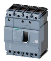
circuit breaker 3VA1 IEC frame 160 breaking capacity class N Icu=25kA @ 415V 4-pole, line protection TM210, FTFM, In=125A overload protection Ir=125A fixed short-circuit protection Ii=10 x In N conductor protection 100% nut keeper kit
