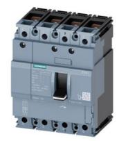
circuit breaker 3VA1 IEC frame 160 breaking capacity class N lcu=25kA @ 415V 4-pole, line protection TM210, FTFM, In=125A overload protection Ir=125A fixed short-circuit protection li=10 x In N conductor protection 50% nut keeper kit
