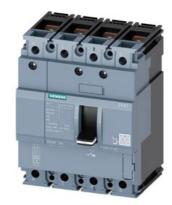
circuit breaker 3VA1 IEC frame 160 breaking capacity class M Icu=55kA @ 415V 4-pole, line protection TM210, FTFM, In=100A overload protection Ir=100A fixed short-circuit protection Ii=10 x In N conductor protection 50% nut keeper kit
