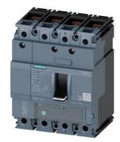
circuit breaker 3VA1 IEC frame 160 breaking capacity class M Icu=55kA @ 415V 4-pole, line protection TM220, ATFM, In=100A overload protection Ir=70A...100A short-circuit protection Ii=10 x In N conductor unprotected nut keeper kit
