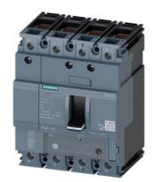
circuit breaker 3VA1 IEC frame 160 breaking capacity class S Icu=36kA @ 415V 4-pole, line protection TM240, ATAM, In=100A overload protection Ir=70A...100A short-circuit protection Ii=5...10 x In N conductor protection 100% clamp connection
