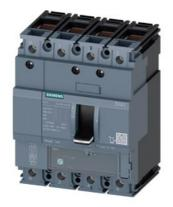
circuit breaker 3VA1 IEC frame 160 breaking capacity class S Icu=36kA @ 415V 4-pole, line protection TM220, ATFM, In=100A overload protection Ir=70A...100A short-circuit protection Ii=10 x In N conductor protection 100% clamp connection
