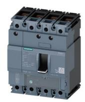
circuit breaker 3VA1 IEC frame 160 breaking capacity class S Icu=36kA @ 415V 4-pole, line protection TM220, ATFM, In=100A overload protection Ir=70A...100A short-circuit protection Ii=10 x In N conductor protection 100% nut keeper kit
