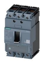
circuit breaker 3VA1 IEC frame 160 breaking capacity class N Icu=25kA @ 415V 3-pole, line protection TM220, ATFM, In=100A overload protection Ir=70A...100A short-circuit protection Ii=10 x In clamp connection
