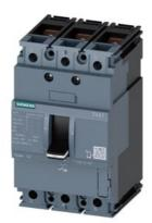
circuit breaker 3VA1 IEC frame 160 breaking capacity class N Icu=25kA @ 415V 3-pole, line protection TM210, FTFM, In=100A overload protection Ir=100A fixed short-circuit protection Ii=10 x In nut keeper kit
