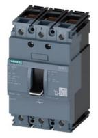
switch disconnector 3VA1 IEC frame 160 3-pole SD100, In=100A without overload protection w/o short-circuit protection clamp connection  $\,$
