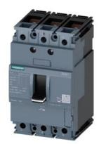
circuit breaker 3VA1 IEC frame 100 breaking capacity class N Icu=25kA @ 415V 3-pole, line protection TM210, FTFM, In=16A overload protection Ir=16A fixed short-circuit protection Ii=20 x In nut keeper kit
