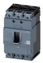
circuit breaker 3VA1 IEC frame 100 breaking capacity class B Icu=16kA @ 415V 3-pole, line protection TM210, FTFM, In=16A overload protection Ir=16A fixed short-circuit protection Ii=20 x In clamp connection
