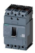
circuit breaker 3VA1 IEC frame 100 breaking capacity class N Icu=25kA @ 415V 3-pole, line protection TM210, FTFM, In=80A overload protection Ir=80A fixed short-circuit protection Ii=10 x In nut keeper kit
