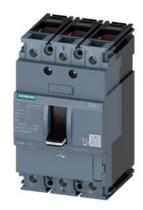
circuit breaker 3VA1 IEC frame 100 breaking capacity class B Icu=16kA @ 415V 3-pole, line protection TM210, FTFM, In=80A overload protection Ir=80A fixed short-circuit protection Ii=10 x In clamp connection
