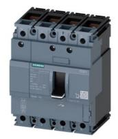
circuit breaker 3VA1 IEC frame 100 breaking capacity class N Icu=25kA @ 415V 4-pole, line protection TM210, FTFM, In=63A overload protection Ir=63A fixed short-circuit protection Ii=10 x In N conductor unprotected nut keeper kit
