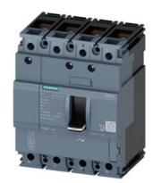
circuit breaker 3VA1 IEC frame 100 breaking capacity class B Icu=16kA @ 415V 4-pole, line protection TM210, FTFM, In=50A overload protection Ir=50A fixed short-circuit protection Ii=10 x In N conductor unprotected nut keeper kit
