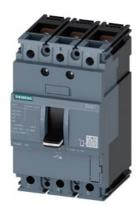
circuit breaker 3VA1 IEC frame 100 breaking capacity class B Icu=16kA @ 415V 3-pole, line protection TM210, FTFM, In=40A overload protection Ir=40A fixed short-circuit protection Ii=10 x In nut keeper kit
