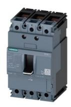
circuit breaker 3VA1 IEC frame 100 breaking capacity class N Icu=25kA @ 415V 3-pole, line protection TM210, FTFM, In=32A overload protection Ir=32A fixed short-circuit protection Ii=10 x In nut keeper kit
