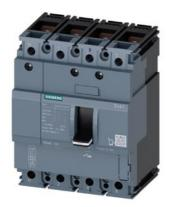
Circuit breaker 3VA1 IEC Frame 100 Switching capacity class B Icu=16 kA @ 415 V 4-pole, system protection TM210, FTFM, In=100 A Overload protection Ir=100 A non-adjustable short-circuit protection Ii = 10 x In N-conductor unprotected Lug terminal
