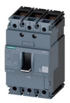
Circuit breaker 3VA1 IEC Frame 100 Switching capacity class B Icu=16 kA @ 415 V 3-pole, system protection TM210, FTFM, In=100 A Overload protection Ir=100 A non-adjustable short-circuit protection Ii = 10 x In Lug terminal
