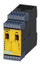
Fail-safe digital module DM-F PROFIsafe, for fail-safe shutdown via bus/PROFIsafe, Us: 110...240 V AC/DC, 2 relay enabling circuits, 2 relay outputs, 3 inputs, maximum achievable SIL IEC 61508: 3, maximum achievable PL ISO 13849-1: E
