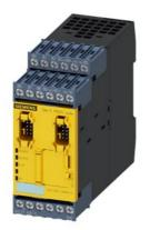
Fail-safe digital module DM-F PROFIsafe, for fail-safe shutdown via bus/PROFIsafe, Us: 24 V DC, 2 relay enabling circuits, 2 relay outputs, 3 inputs, maximum achievable SIL IEC 61508: 3, maximum achievable PL ISO 13849-1: E
