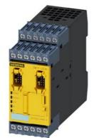
Fail-safe digital module DM-F local, for fail-safe shutdown via hardware signal Us: 24 V DC 2 relay enabling circuits, 2 relay outputs, safety function can be set via DIP switch, maximum achievable SIL IEC 61508: 3, maximum achievable PL ISO 13849-1: E
