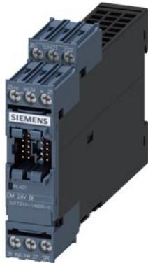
Digital module, 4 inputs and 2 relay outputs, input voltage 24 V DC, relay outputs bistable, max. 2 digital modules, for SIMOCODE pro V basic unit
