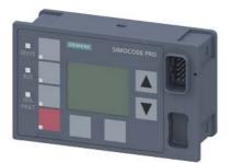
Operator panel with display for SIMOCODE pro V, installation in control cabinet door or front plate, can be plugged onto basic unit or extension modules, 7 LEDs for status display and 4 freely assignable keys for manual control, Color: titanium gray
