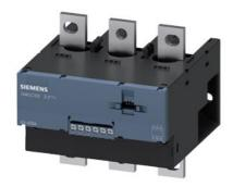
Current/voltage measuring module for dry-running protection of centrifugal pumps in hazardous areas; set current 63 ... 630 A, voltage measurement up to 690 V, width 145 mm, busbar connection
