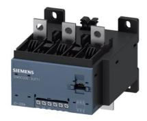
Current/voltage measuring module for dry-running protection of centrifugal pumps in hazardous areas; set current 20 ... 200 A, voltage measurement up to 690 V, width 120 mm, busbar connection
