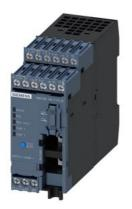
Basic unit SIMOCODE pro V PN GP Ethernet/PROFINET IO, PN system redundancy, OPC UA server, Web server, transmission rate 100 Mbps, 2 x bus connection via RJ45, 4 I/3 Q freely parameterizable, Us: 110...240 V AC/DC, input for thermistor connection Monostable relay outputs, expandable by 1 extension module(DM, TM, EM)
