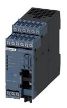
Basic unit SIMOCODE pro V PN GP , Ethernet/PROFINET IO, PN system redundancy, OPC UA server, Web server, transmission rate 100 Mbps, 1 x bus connection via RJ45, 4 I/3 Q freely parameterizable, Us: 24 V DC, input for thermistor connection Monostable relay outputs, expandable by 1 extension module(DM, TM, EM)
