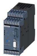
Basic unit SIMOCODE pro V PB PROFIBUS DP interface 12 Mbit/s, RS 485, 4I/30 freely parameterizable, Us: 24 V DC, input for thermistor connection Monostable relay outputs, expandable by extension modules
