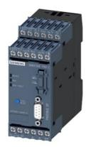
Basic unit SIMOCODE pro C, PROFIBUS DP interface 12 Mbit/s, RS 485, 4I/3O freely parameterizable, Us: 110...240 V AC/DC, input for thermistor connection Monostable relay outputs
