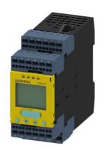
SIRIUS safety relay Safety-oriented Speed monitoring 24 V DC, 45 mm overall width Spring-type terminal EC instantaneous: 2 NO EC delayed: 0 SC: 2 electrical Auto-start/manual start Basic device Maximum achievable PL according to EN 13849-1: e Maximum achievable SIL according to IEC 61508: 3
