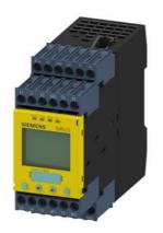
SIRIUS safety relay Safety-oriented Speed monitoring 24 V DC, 45 mm overall width Screw terminal EC instantaneous: 2 NO EC delayed: 0 SC: 2 electrical Autostart/manual start Basic device Maximum achievable PL according to EN 13849-1: e Maximum achievable SIL according to IEC 61508: 3
