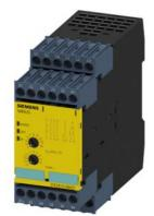
SIRIUS safety relay safety-oriented Standstill monitoring 24 V DC, 45 mm screw terminal EC instantaneous: 3 NO + 1 NC EC delayed: 0 SC: 3 Auto-start Basic unit max. error category EN 954-1: 4 Maximum achievable PL according to EN 13849-1: Maximum achievable SIL according to IEC 61508: 3
