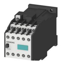
Contactor relay, 55E, EN 50011, 5 NO + 5 NC, screw terminal, DC operation, 24 V DC
