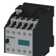
Contactor relay, 55E, EN 50011, 5 NO + 5 NC, screw terminal, AC operation, 230 V AC 50/60 Hz
