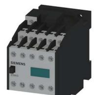
Contactor relay, 55E, EN 50011, 5 NO + 5 NC, screw terminal, AC operation, 24 V AC 50/60 Hz
