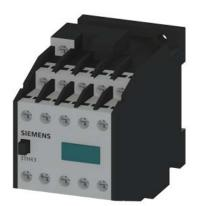
Contactor relay, 73E, EN 50011, 7 NO + 3 NC 1U screw terminal AC operation, 110 V AC 50/60 Hz
