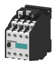
Contactor relay, 44E, DIN EN 50011, 4 NO + 4 NC, screw terminal AC operation 110 V AC 50 Hz/132 V AC 60 Hz
