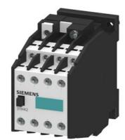
Contactor relay, 71E, DIN EN 50011, 7 NO + 1 NC, screw terminal AC operation 24 V AC 50/60 Hz
