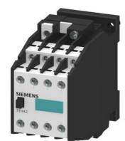
Contactor relay, 62E, DIN EN 50011, 6 NO + 2 NC, screw terminal AC operation 230/220 V AC 50 Hz, 276/264V 60Hz
