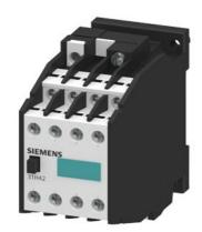
Contactor relay, 62E, DIN EN 50011, 6 NO + 2 NC, screw terminal AC operation 220 V AC 50/60 Hz
