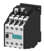
Contactor relay, 62E, DIN EN 50011, 6 NO + 2 NC, screw terminal AC operation 42 V AC 50/60 Hz
