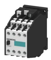
Contactor relay, 53E, DIN EN 50011, 5NO + 3NC, screw terminal AC operation 220 V AC 50/60 Hz
